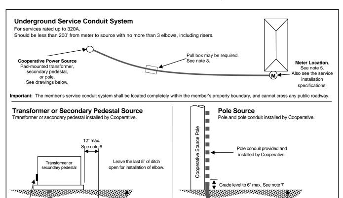
recommends that all electrical work be done by a qualified, licensed electrical contractor.The member shall provide and install all secondary conduit; conduit shall have an 80lb non-metallic pull line installed. See table below for conduit diameter. Consult Cooperative for service above 320A.
