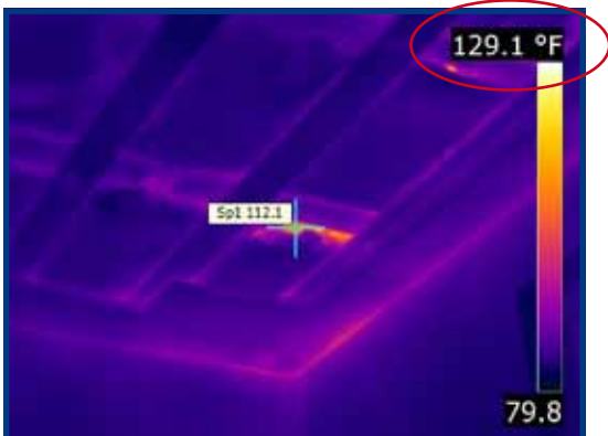
An infrared camera detects heat nearing 130 degrees. The heat is moving from a hot rooftop through improperly installed fiberglass insulation into an air-conditioned dwelling.
